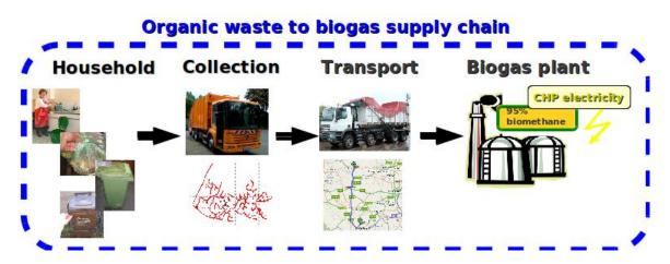
Figure 16 Typical elements of a food waste to biogas supply chain. All processes and raw material are carried out and sourced locally.
